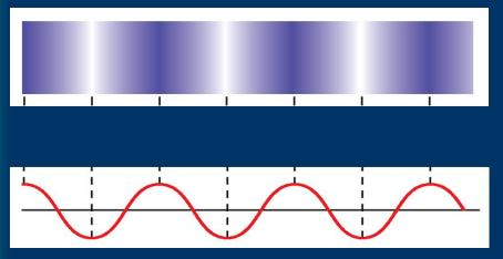
The diagram shows compressions (dark) and rarefactions(white). If you measured the pressure or density of the air and plotted these against position, how would the graph appear?
