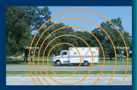
• The *Doppler effect* is the observed change in frequency due to the motion of the source or observer.
